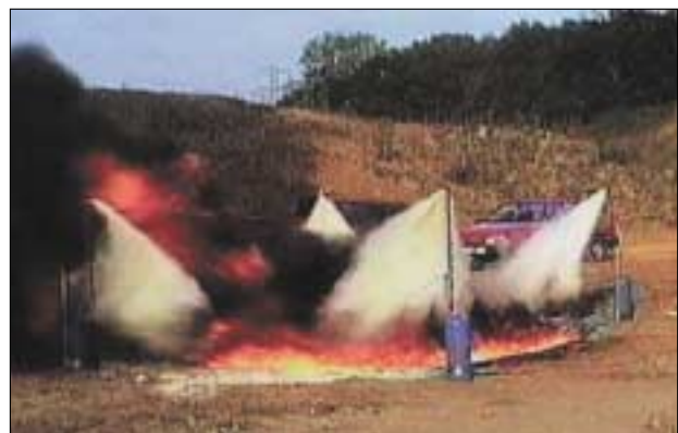
Any number of Firetrace extinguishers can be linked to discharge simultaneously
