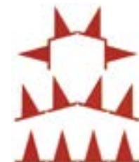
Prikka Brick strip installation options
