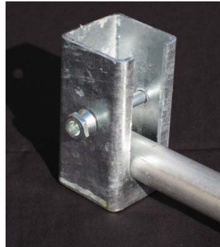
Alley Bracket showing the shaft in place and the shaft retaining bolt with shear nut.
